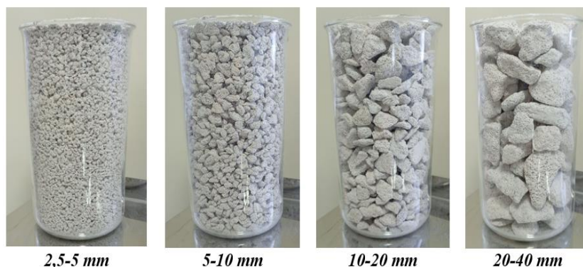
Fig. 2. Packing density of different fractions of autoclaved porous aggregate
