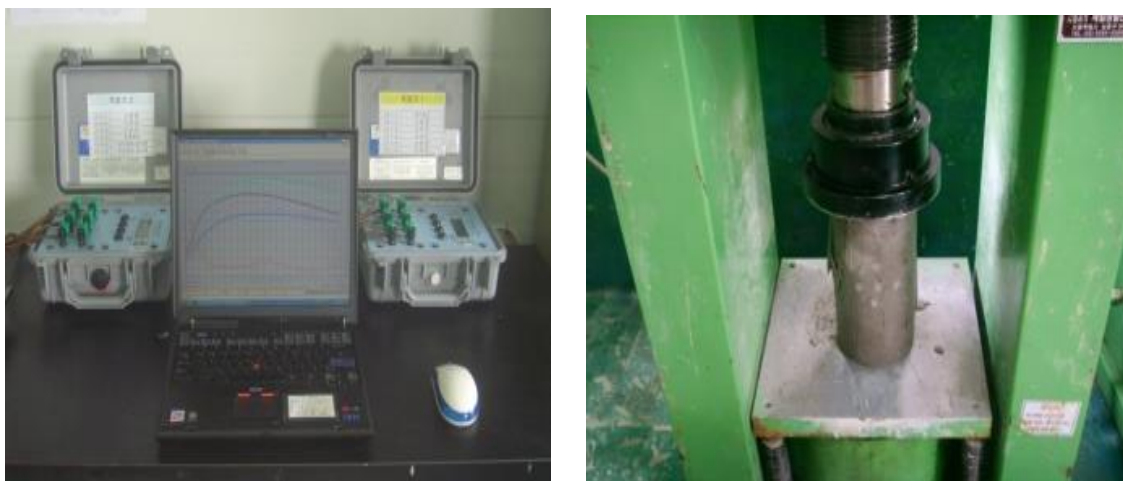
Photo 2. Monitoring of heat of hydration and compressive strength testing with cylindrical specimens
