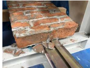
Figure 8. Failure mode of control specimen [31]
