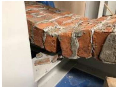
Figure 8. Failure mode of control specimen [31]
