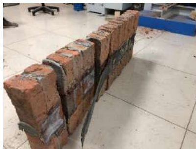
Figure 9. Failure mode of S-S1-L1 [31]
