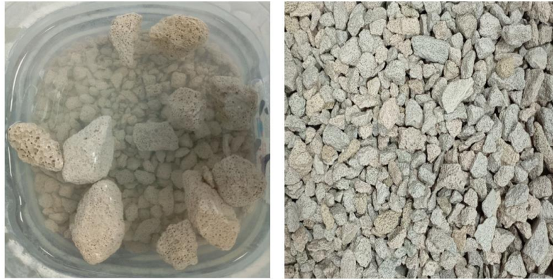
Fig. 5. Photographs taken during the study of water absorption characteristics of autoclaved porous aggregate
