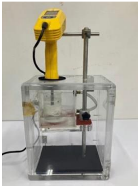
Fig. 6. An ultrasonic homogenization apparatus [from Atmaca et al. [4] with permission from Springer]
