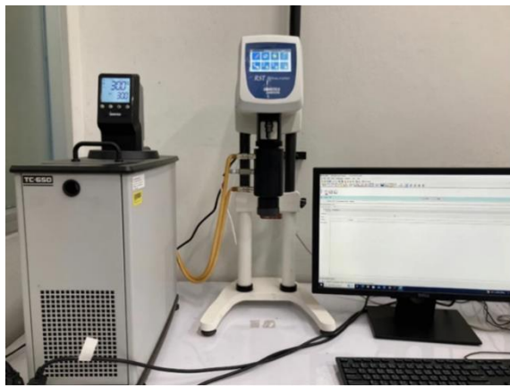
Fig. 13. Experimental setup for viscosity measurement [from Dalkilic et al. [11] with permission from Elsevier] (a) and comparison of measured data with reference one [6] (b)
