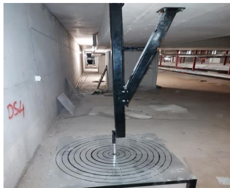
Figure 11. Displacement measuring device located at the isolation story of Osmaniye State Hospital [12]
