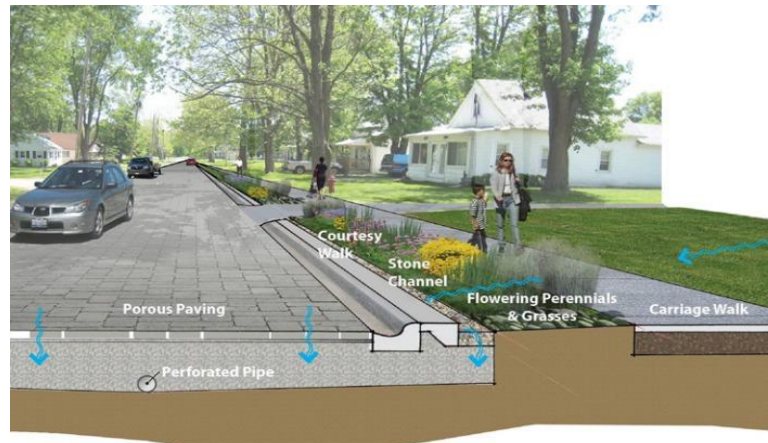
Figure 1. How the infrastructure (green drainage system to reuse surface water) interacts with the superstructure (permeable surfaces, porous pavement) in an optimal sustainable green space Source: The Sustainable Sites Handbook, Meg Calkins, 2012 [12]
