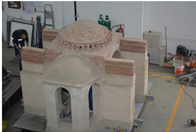
Figure 10. Scaled model of Hagia Sophia on the shake table (Kasimzade et al., 2018)
