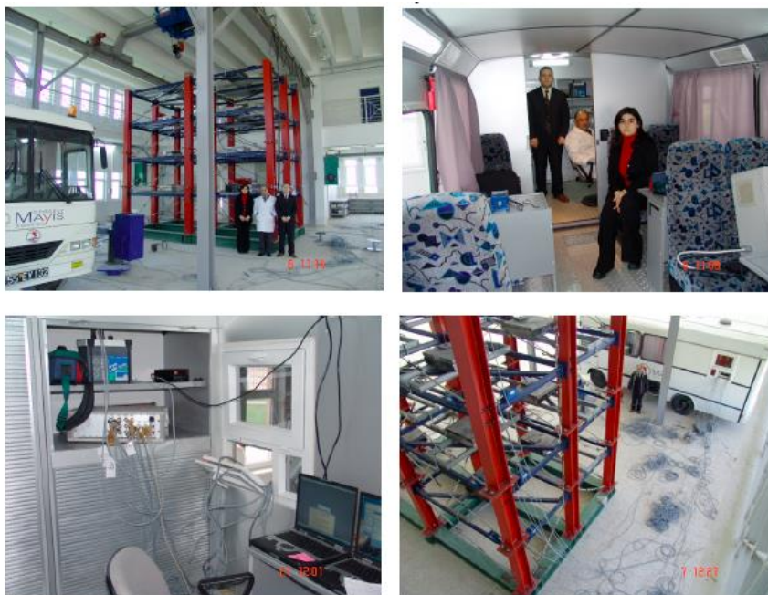
Figure 5. Mobile structural monitoring system, steel frame benchmark structure, outside and inside of the mobile laboratory (Kasimzade Archive, (Kasimzade et al., 2006,2007,2012)
