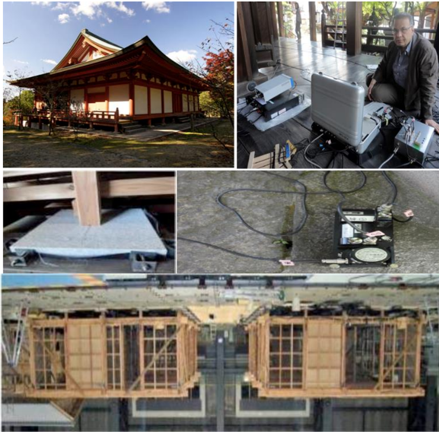
Figure 7. a) Wooden structure; b) Response measurement and evaluation; c) Structure support modelling for test model; d) Layout of the reference device; e) Test model of structure (Kasimzade Archive)
