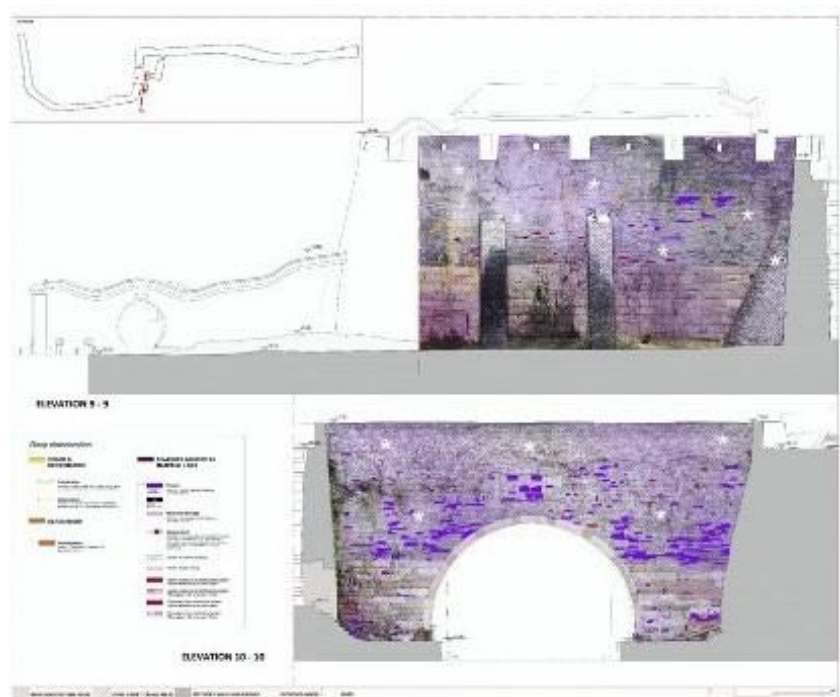
Figure 43. One of the decay analysis and restoration project boards on an orthophoto
