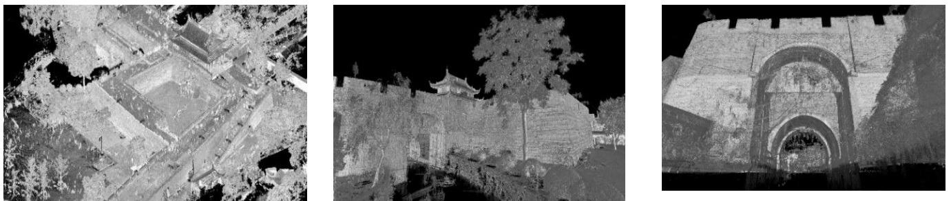
Figure 34, 35, 36. The laser-scanner survey of the Panmen area
